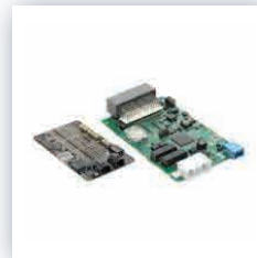
Battery Management System
